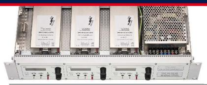
© iseg Spezialelektronik GmbH 19" THQ device equipped with three DPS high voltage modules
