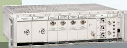
CPS 3U-eurocassette modules in a digitally controllable 19" crate © iseg GmbH
