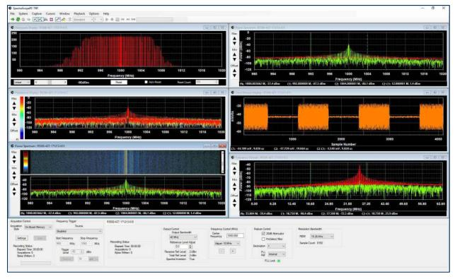
SpectraScopeRT is a Windows based spectrum analyzer application that requires no programming and allows for integrated operational control of both the RF Downconverter receiver and the Digitizer for signal capture, analysis, recordings.
