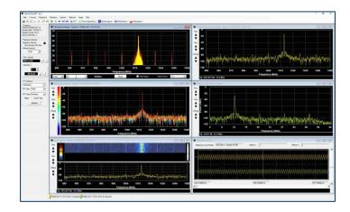
Playback operations utilize familiar navigation toolbar buttons for starting playback, stopping playback, stepping backwards and forwards, and moving back to start.
