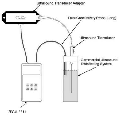
Typical Electrical Leakage Test
